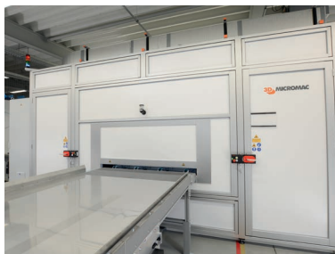
Example of handling table, fully automated substrate transfer into machine
